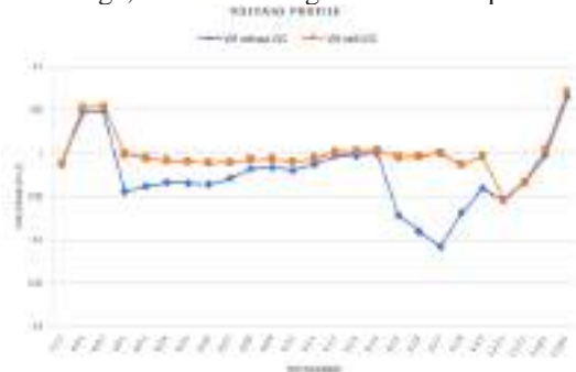
Fig. 8: Voltage profile of remaining 25 bus with and without SVC
