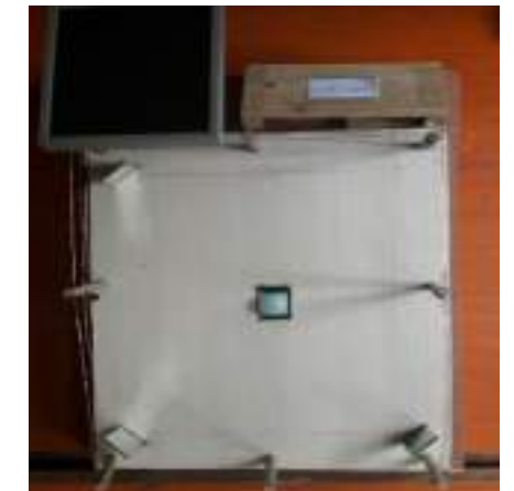
Figure 2: Fabricated model of alarm fencing and light footpath sensor.
